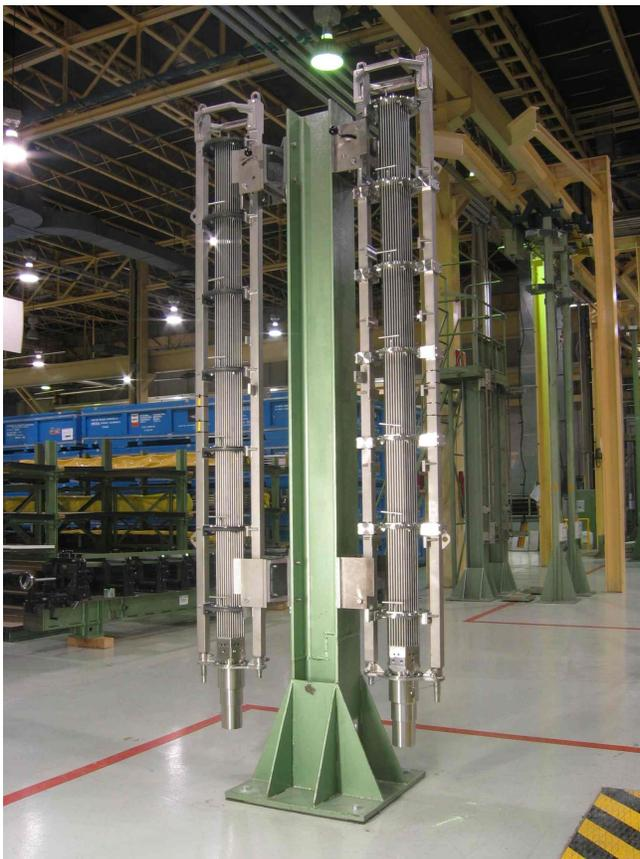
*Two Lead Test Assemblies of the NOVA E-3 design
